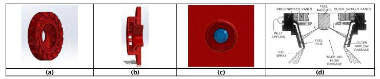
**Figure 2.** Inflow swirler showing: (a) one of the radial swirling inflow vanes, (b) side-view of the swirler cut-out without the center-body atomizer, (c) top view of center-body air blast atomizer (blue), and (d) side view of swirler showing swirler vanes, fuel injector, and spray.
