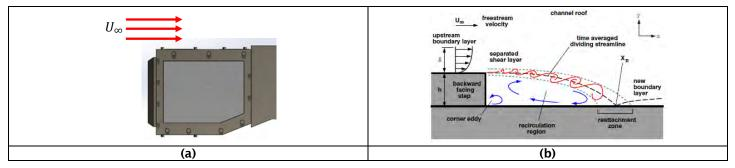
**Figure 4.** Physics of "stepped" quench hole design showing: (a) transverse flow over the liner coming to the quench, and (b) flow physics at a backward facing step.
