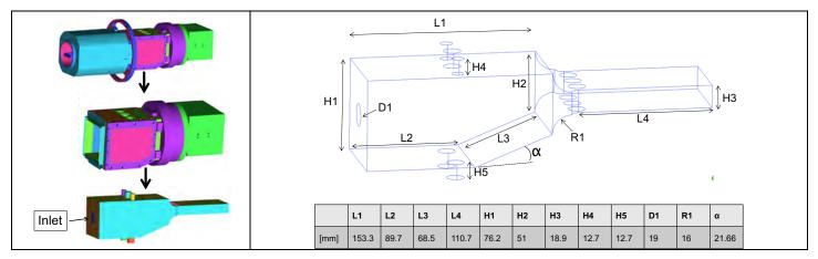
**Figure 8.** Initial computational domain used for the GT experiment simulation. Left: reduction from experiment CAD model to computational CAD model. Right: dimensions of computational domain.
