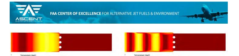
Figure 19. Snapshot of temperature field for two different frequencies. Left: lower frequency. Right: higher frequency.
