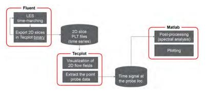
**Figure 16.** Analysis workflow from using Ansys Fluent for simulation to Tecplot for post-processing and visualization to Matlab for final transfer function calculation.
