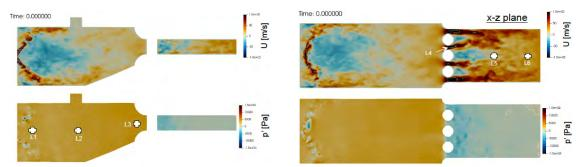
**Figure 9.** Snapshots of the velocity (top) and pressure fluctuations (bottom) in a cut-plane passing vertically through the center of the swirler (left) and in a cut-plane passing horizontally through the center of the exhaust section (right).
