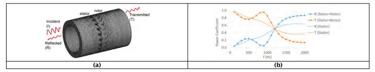
Figure 20. (a) Ideal wave simulation mesh. (b) Predicted sound power coefficients as a function of frequency.
