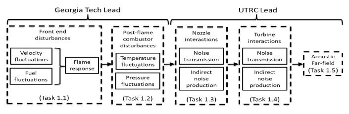
Figure 1. Physical processes and project tasks for noise generation.
