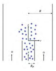
Figure 10. Schematic of the ducted spray flame configuration. Fuel droplets are injected in the center duct (shown in blue) and oxidizer gas is injected in the outer ducts.
