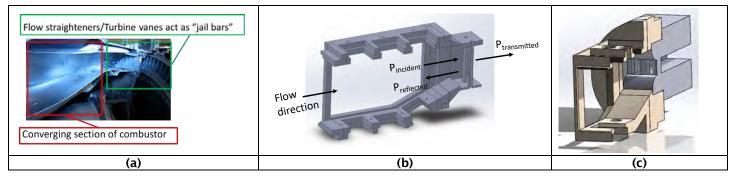
**Figure 5.** (a) Cross-section from a real engine showing converging section and array of turbine vanes, (b) cross-section from GT design showing converging section followed by, (c) "jail bars" to mimic turbine vanes.
