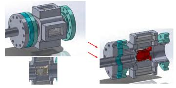
Figure 7. Placement of combustion liner inside the pressure vessel at the GT combustion lab.
