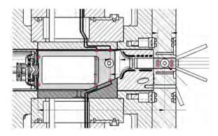
Figure 12. Cut-away of the RTRC experiment showing side view with the inflow in the left, combustion zone, convergent section, followed by bell mouth feature before jail bars. Pressure tap locations shown in red.
