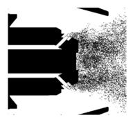
Figure 13. Snapshot of droplets and atomization from baseline production simulation. Spray is seen to remain in the core with minimal wall filming.
