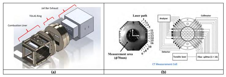
**Figure 6.** (a) Exploded view showing combustion liner, TDLAS, and jail bar exhaust system in the GT rig, (b) TDLAS probe array in the ring.
