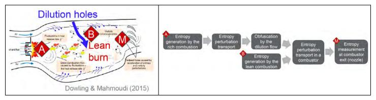
**Figure 15.** Mechanism of entropy wave generation and transport in combustor. Left: aeroengine combustor showing different regions with generation and transport. Right: flow chart for modeling and understanding entropy wave transport through simulation.
